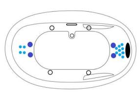
23 Jet Whirlpool(3) 115v 20AMP GFCI Circuits2 Motor Access Locations
